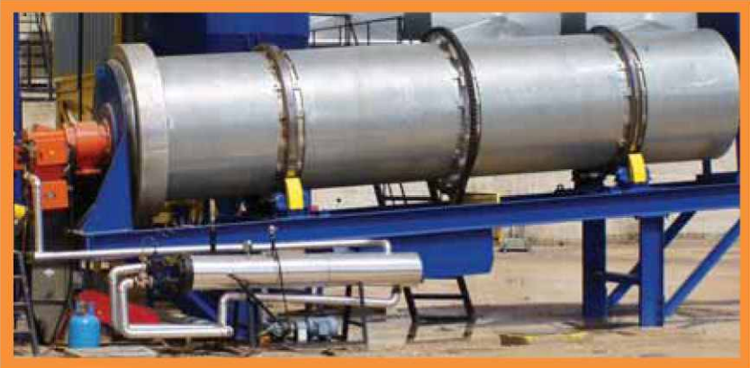
Hot Oil Heat Exchanger
