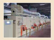
Gazoram Process Burner is used in not only new dryer, Also they are used in conversion of steam or hot oil dryers.
