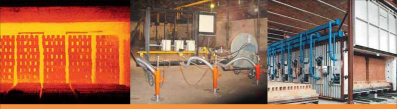
In brick drying ovens the damp product which has to be homogene dry in an optimum period, the water inside of the product has to be vaporized. Wrong design of the drying-heating system is causig of blowing up, cracking, splitting of the product during the heating process. The product will be not resistant. Therefore, every row material needs special engineering calculations, experience and automation system.
